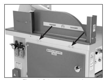
Figure 8. Bolts to be removed.
